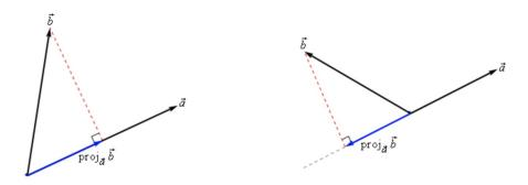
parallel to  $\overrightarrow{a}$ , starts at the same point both of the original vectors started at and ends where the dashed line hits the line parallel to  $\overrightarrow{a}$ .
