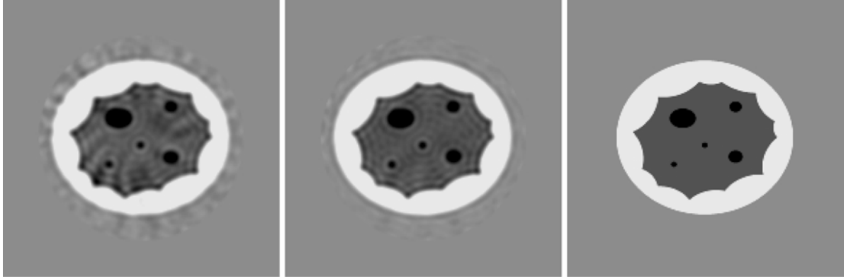
Adjoint Methods as Applied to Inverse Problems, Fig. 1 Reconstruction of breast phantom from 32 sources at 100 kHz. Left: after 3 sweeps. Middle: after 6 sweeps. Right: original
