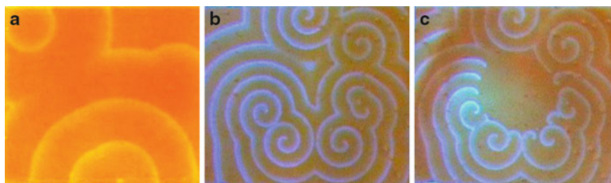
Belousov–Zhabotinsky Reaction, Fig. 1 Light controls wave behavior in the light-sensitive BZ reaction (a) showing circular waves in the excitable light-sensitive BZ reaction; (b) the reaction is subsequently illuminated with a blue LED (355 nm)
