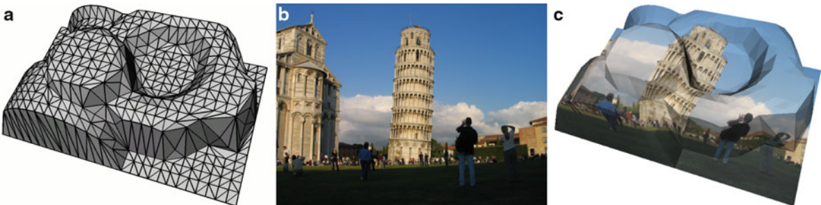
Geometry Processing, Fig. 7 The parameterization of a triangle mesh (a) over the plane can be used to map a picture (b) onto the surface of the mesh (c). This process is called texture mapping and is supported by the graphics hardware
