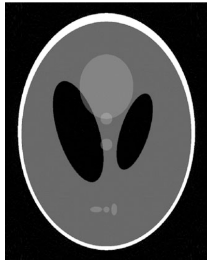
Medical Imaging, Fig. 3 Filtered back-projection reconstruction of the Shepp–Logan phantom from the data in Fig. 2
