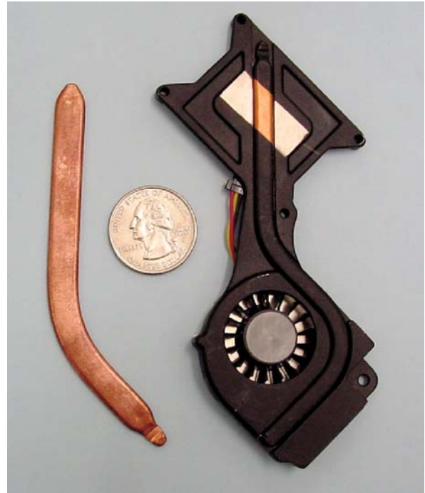
Micro Heat Pipes, Figure 10 Miniature heat pipes in a laptop computer cooling
