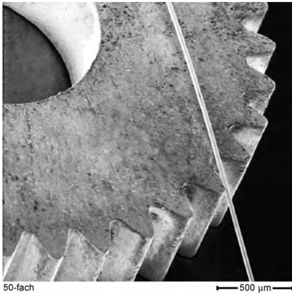
Micromolding (Injection and Compression Molding), Figure 7 SEM image taken of a micromachined part created through wire-EDM process (taken from [14])
