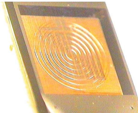
Thermopneumatic Valve, Figure 1 Thermopneumatic actuator consisting of a corrugated p+ silicon diaphragm as the residual stress relaxation structure and a microheater for thermopneumatic actuation [4]
