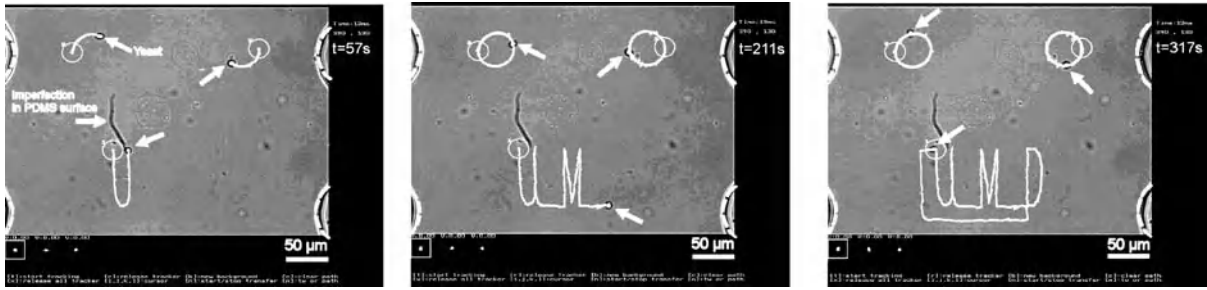
Control of Micro-Fluidics, Figure 4 Steering of 3 yeast cells (5 \mu\text{m} diameter, Red Star, Giant Food) with small surface charge (electrophoretic mobility c = (-23.3 \pm 6.9)10^{-9} \text{ m}^2\text{V}^{-1}\text{s}^{-1} ) around two circles and a 'UMD' path (for 'University of Maryland'). The yeast cells are visible as small black dots with a white center (the three target cells are marked with a white arrow in each image), and the white curves are the trajectories that the target cells have traced out. The three beads are being steered to within an accuracy of one pixel (corresponding to less than 1 \mu\text{m} )
