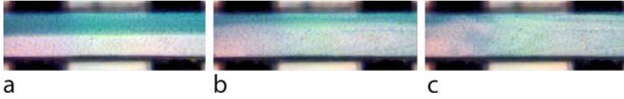
Electrokinetic/ElectroHydrodynamic Flow Instability, Figure 3 Electrohydrodynamic mixing in a DC electric field. The images show the outlet branch of the microchannel after the device has been loaded with two fluids. (a) The initial condition showing a dark green fluid which corresponds to a doped and dyed oil while the clear fluid represents the pure oil. (b) The mixture after the application of an electric field E = 4 \times 10^5 V/m. (c) Electric field intensity of E = 6 \times 10^5 V/m. Images taken from [8]
