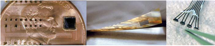
Micro- and Nanoscale Anemometry: Implication for Biomedical Applications, Figure 10 (a) Top view of transparent parylene skin with Au wires connected to a single silicon island. (b) Side view of flexed parylene skin with Au wires and silicon island. (c) Flexed parylene skin with platinum (Pt) wires
