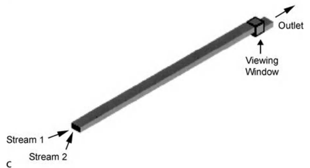
Passive Micromixers, Figure 6 (a) Schematic of the three-dimensional serpentine channel. “Viewing windows” in the channel are labeled 1–10. (b) Schematic of zigzag channel. (c) Schematic of straight channel [9]
