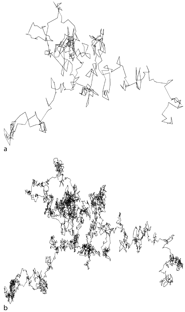
Fundamentals of Diffusion in Microfluidic Systems, Figure 1 Simulated paths of a Brownian particle. (a) Path recorded on a large timescale and (b) same path recorded on a smaller timescale. More details emerge as we use smaller time scales
