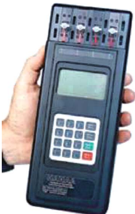
Lab-on-Chip Devices for Biodefense Applications, Figure 3 The Handheld Advanced Nucleic Acid Analyzer from Lawrence Livermore National Laboratory
