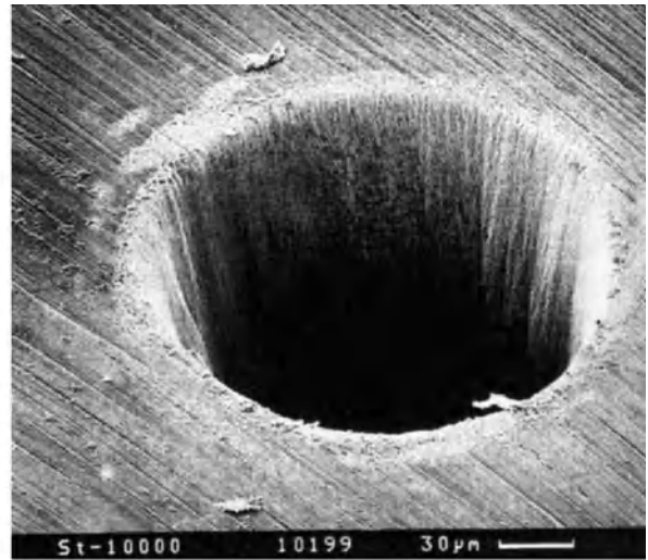
Laser Ablation, Figure 1 (a) Nanosecond-pulse laser ablation of a hole in a 100 mm thick steel foil with a pulse width of 3.3 ns, fluence of 4.2 \text{ J/cm}^2 at a laser wavelength of 780 nm. (b) Femtosecond laser ablation of a hole in a 100 mm thick steel foil with a pulse width of 200 fs, fluence of 0.5 \text{ J/cm}^2 at a laser wavelength of 780 nm
