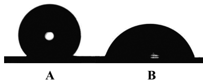
Figure 7.2. Wetting transitions observed by vibration of a 15\ \mu\text{l} water drop deposited on a micrometrically rough PDMS surface. A: the initial Cassie state; B: the Cassie impregnating state induced by vibrations.
