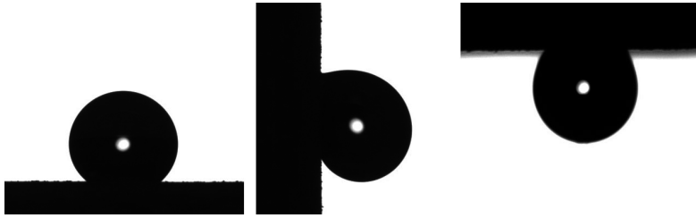
Figure 6.9. A 10\ \mu\text{l} water droplet deposited on a surface built of lycopodium particles.
