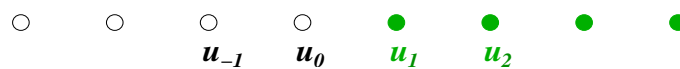
Figure 11.4: An illustration of the eliminated and retained degrees of freedom. The degrees of freedom associated with the filled circles are kept. Others are eliminated.
