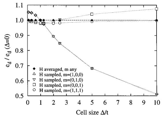
FIG. 2. Computed demagnetization energy as a function of cell size for a uniformly magnetized 5 : 1 : 0.1 rectangular particle. Cell size is expressed relative to particle thickness  $t$ . The energy is calculated using either sampled demagnetizing fields (open symbols) or averaged demagnetizing fields (solid diamonds).
