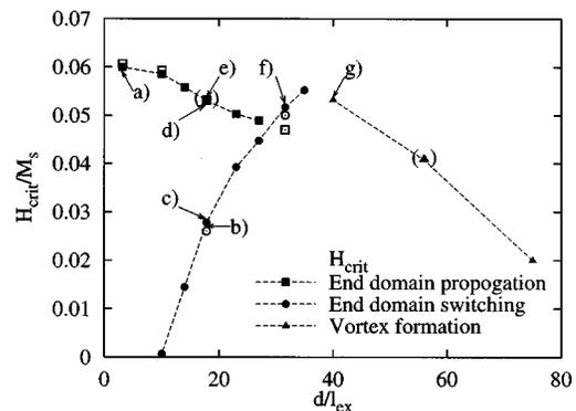
FIG. 4. Critical fields for  $\mu$ MAG standard problem No. 2 as a function of reduced particle width  $d/l_{ex}$ . The symbol size is approximately equal to the uncertainty in  $H_c/M_s$  due to the field step size. Filled and open symbols are results obtained using the constant magnetization and constant charge methods, respectively. Superimposed data points are enclosed by parentheses. Labels a–g correspond to magnetization patterns displayed in Fig. 3
