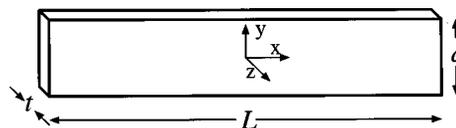
FIG. 1. The geometry of  $\mu\text{MAG}$  standard problem No. 2, a 0.1:1:5 aspect ratio rectangular block of magnetic material with exchange energy, magnetostatic energy, and Zeeman energy only.
