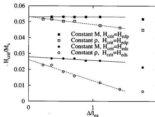
FIG. 5. Critical fields for  $\mu$ MAG standard problem No. 2 as a function of normalized cell size  $\Delta/l_{ex}$  with  $d/l_{ex} = 17.8$ . Squares indicate end domain propagation fields ( $H_{edp}$ ) and circles indicate end domain switching fields ( $H_{eds}$ ). Filled and open symbols are results obtained using the constant magnetization and constant charge methods, respectively.
